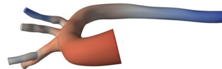
Pressure field inside aorta gen. with CFD.
