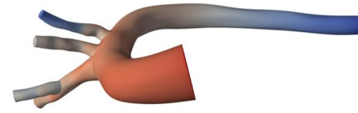
Pressure field inside aorta gen. with CFD.
