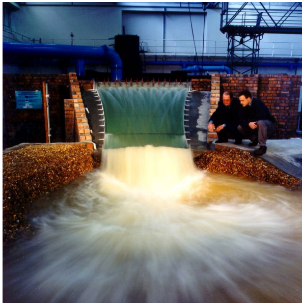
Caption: Prof Albert Rooseboom (left) with Dr Andre Bester (former DWS) during one of his last major model studies at the laboratory (1998–1999). The 1:60 scale model of the Maguga Dam in Swaziland featured a labyrinth spillway, designed for a discharge capacity of 11,000 m 3 /s.
