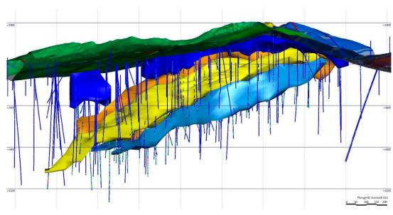
3D Block Model, showing drill holes sampling points for characterisation
