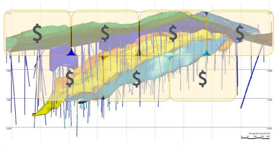
Simplistic illustration of geometallurgical domains, associated with dollars and cents
