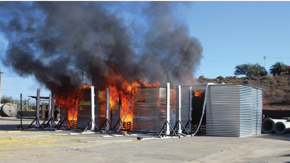
Large-scale fire test on three informal settlement dwellings, as part of a PhD study by Antonio Cicione.
