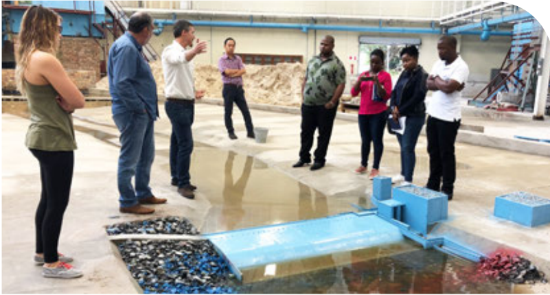
In the Hydraulic Laboratory: Prof Gerrit Basson (third from the left) explains the hydraulic model tests of the Mhlathuze weir at Richards Bay to the client, Mhlathuze Water, during 2018.
