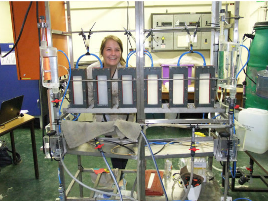
Master's student Marielle Hurter with the test unit that she constructed for the evaluation of hydraulic flux and concentration polarisation behaviour in forward osmosis systems.
